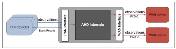
Figure 42 : Model showing how AHD may collect observations from multiple PAN devices at any given point in time and a single PAN device may deliver data to multiple persistent sessions. Likewise, an AHD may deliver these observations to zero or more WAN devices.
