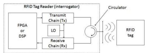
Figure 15 : Typical RFID Reader / Tag system (source: National Instruments 2010)
