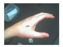
RFID tag for implant into human hand
