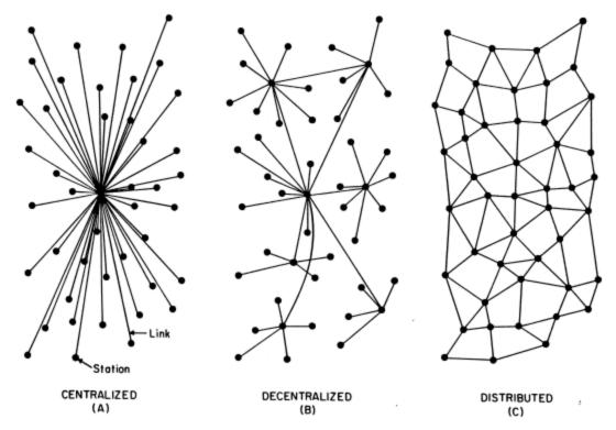
Figure 25 : showing centralised, decentralised and a distributed P2P network<sup>14</sup>
