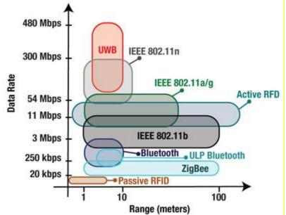
Figure 22 : Showing distribution of various communication protocols data rate and range<sup>12</sup>
