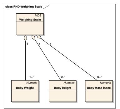
Figure 40 : Object model for Weighing Scale following IEEE 11073-10415:2008
