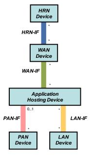
Figure 43 : Continua Topology (from Continua Design Guidelines V1.5)
