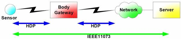
Figure 7 : Data exchange (Bluetooth HDP) between medical sensor, BAN/PAN and transcending WAN together with major associative protocol linkage to IEEE11073<sup>6</sup>.
