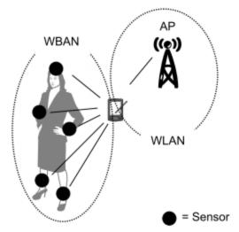
Figure 13 : Extending WBAN range using WLAN
