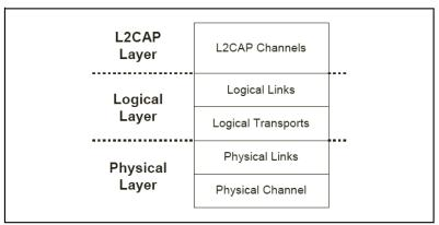
Figure 4 : Bluetooth generic data transport architecture
