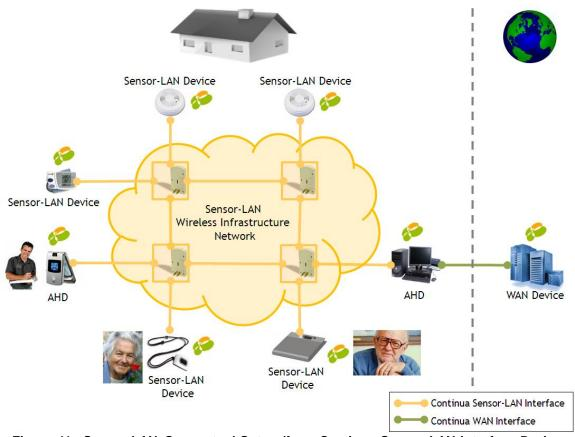
Figure 41 : Sensor-LAN Conceptual Setup (from Continua Sensor LAN Interface Design Guidelines)
