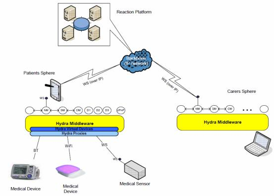
Figure 35 : Incorporation of devices using the Hydra middleware.
