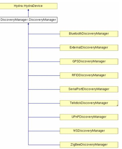
Figure 38 : The dedicated discovery module in Hydra Discovery Manager that handles separate device protocols.
