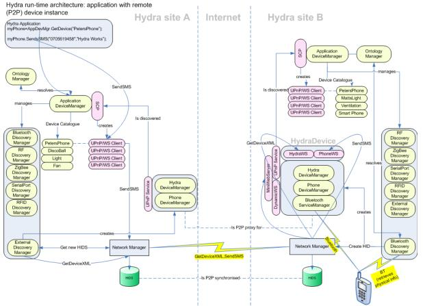
Figure 36 : Hydra run-time P2P architecture.
