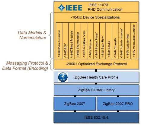
Figure 9 : ZigBee Health Care architecture
