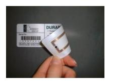
RFID tag with antenna, printed on a barcode label
