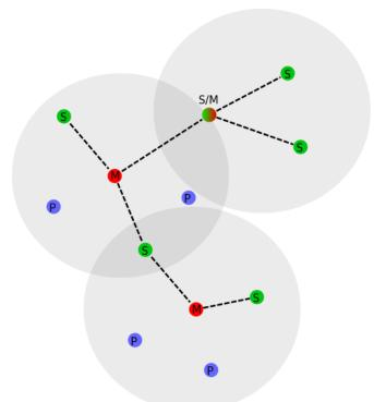
Figure 3 : Example of Bluetooth network topology (M: Master, S: Slave, P; Parked)
