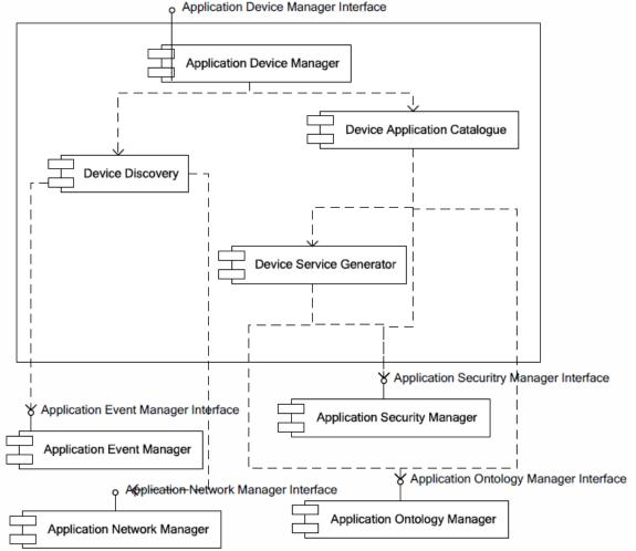
Figure 37 : showing the Hydra Application Device Manager interface with underlying relationships.
