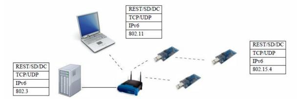
Figure 24 : RESTful supports multiple link layers and with seamless network bridging, the sensor networks become a natural part of the IP network
