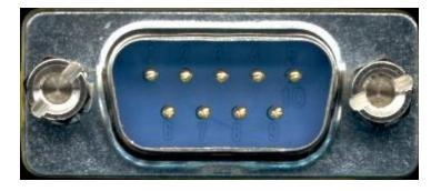
Figure 20 : D-sub 9 connector pinout
