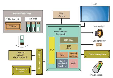
Figure 27 : Example of a home glucose meter circuit with microcontroller<sup>16</sup>.
